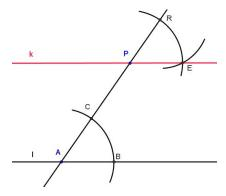
1. Construct a line through P parallel to [AB].
