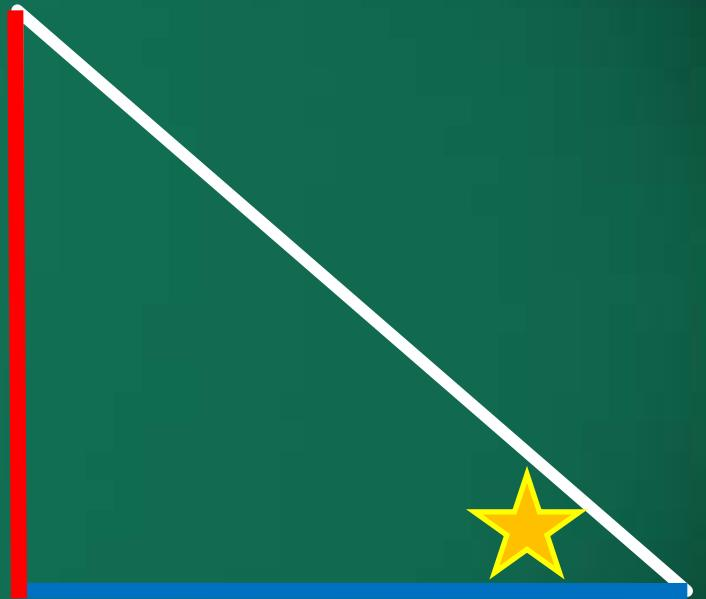
$$\frac{\text{height of building}}{\text{length of building shadow}} = \frac{\text{my height}}{\text{length of my shadow}}$$
